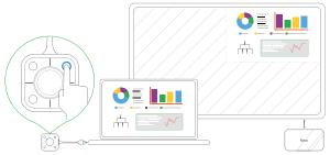
Press any corner button on the LauncherOne to project your computer's screen onto the corresponding quadrant of the display.
