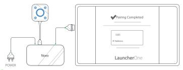
③ Wait for the main and corner buttons on the LauncherOne to light up blue and the Pairing Completed screen to be shown on the display.
