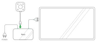
1 Connect the LauncherOne to the NovoConnect device.
